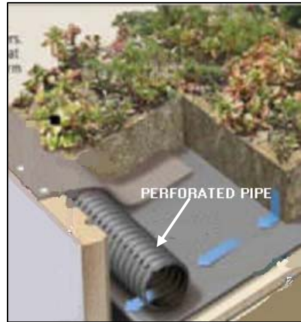
Figure 25. Perforated Pipe between Insulation and Filter Fleece Layers Source: Carey
